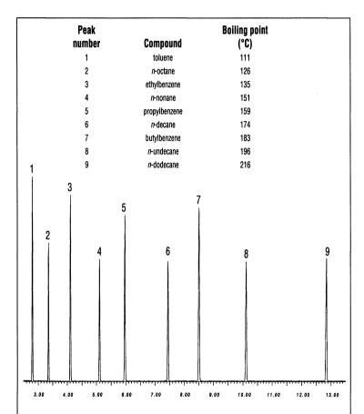
**Figure 1.** Boiling point elution order for homologous series. Column, DB-1 30 m  $\times$  0.25-mm i.d. (0.25- $\mu$ m film thickness); split injector, 250°C; 1:50 split ratio; MS detector, full scan m/z 40–200; 280°C transfer line; helium carrier gas, 32 cm/s; column temperature, 50–120°C at 5°C/min.
